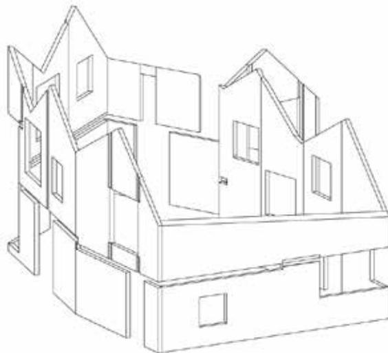
All internal walls and ceilings consist of the exposed timber structure. Where doors are required in timber walls, they are built to match the thickness and finish to create a continuity of material feel and appearance. Space is optimised by integrating fittings, wardrobes and the fireplace into the timber walls. Limestone tiling for the bathrooms is colour-matched to the exposed timber so that there is little visual distinction between them and the rest of the house.
