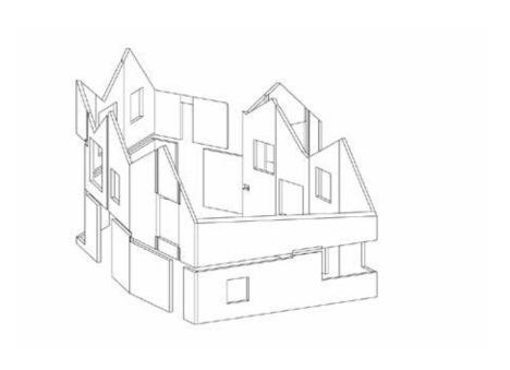
All internal walls and ceilings consist of the exposed timber structure. Where doors are required in timber walls, they are built to match the thickness and finish to create a continuity of material feel and appearance. Space is optimised by integrating fittings, wardrobes and the fireplace into the timber walls. Limestone tiling for the bathrooms is colour-matched to the exposed timber so that there is little visual distinction between them and the rest of the house.
